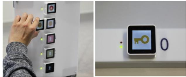
**Figure 3: LiftACube with self-made sensor board with 5 high positions for Sifteo Cubes and 1 position for the free cube.**
