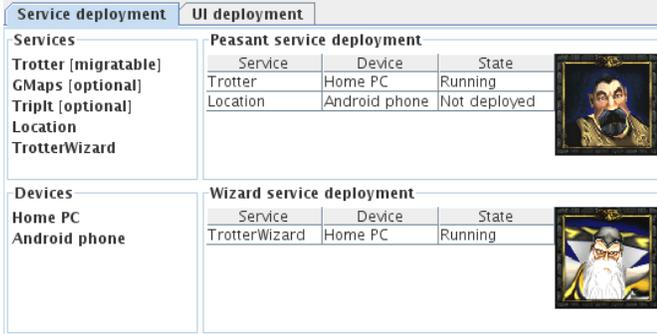
Fig. 5. Generating a deployment descriptor to configure the distribution of peasant and wizard services.
