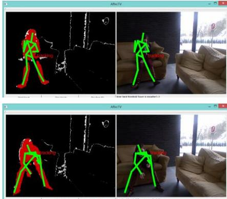
Figure 3 Screenshots of posture capturing software optimized for sitting postures using depth camera.
