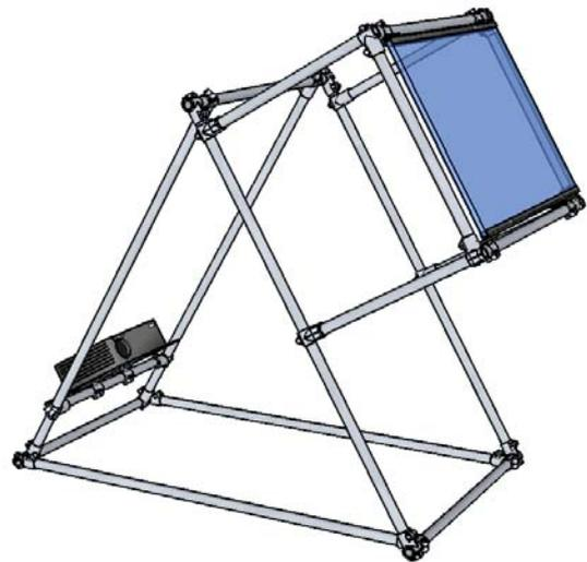
Figure 1: Setup of the multi touch table
