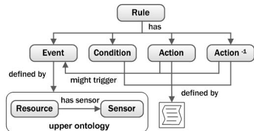
Fig. 3. The behavior of an application is described using  $ECAA^{-1}$  rules.
