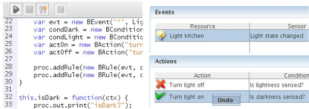
Fig. 6. A script connects a SunSPOT device with a light resource through behavior rules. The events that are fired and the actions that are executed by the rule engine as a reaction to these events can be monitored and undone.
