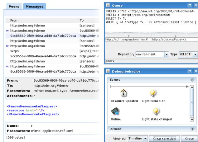
Fig. 1. Tools add live inspection capabilities to pervasive applications such as monitoring the messages that are exchanged between resources, querying the current state of the environment and observing the behavior of running applications.
