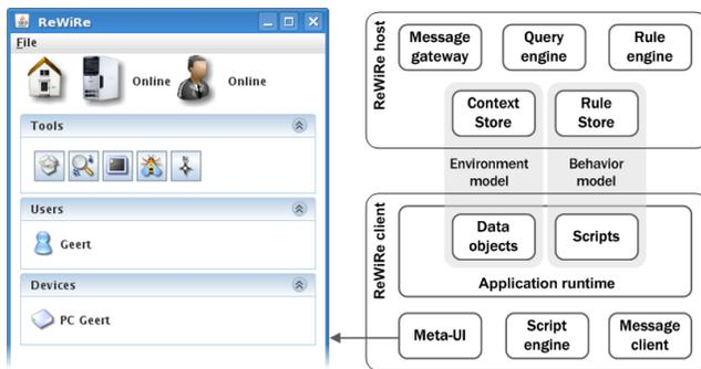
Fig. 4. Environment and behavior models span a host platform and client platforms installed on heterogenous devices. A meta-user interface integrates debug tools for pervasive applications such as those listed in figure 1.
